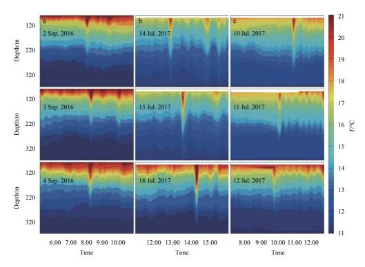
**Fig. 1.** Water temperature profiles of three types of ISWs signatures observed by thermistor chain attached to the mooring deployed in the west of Dongsha Islands in the SCS from 30 June 2016 to 21 July 2017. a. Type-a ISW signatures, b. Type-b ISW signatures, and c. newly observed Type-c ISWs.
